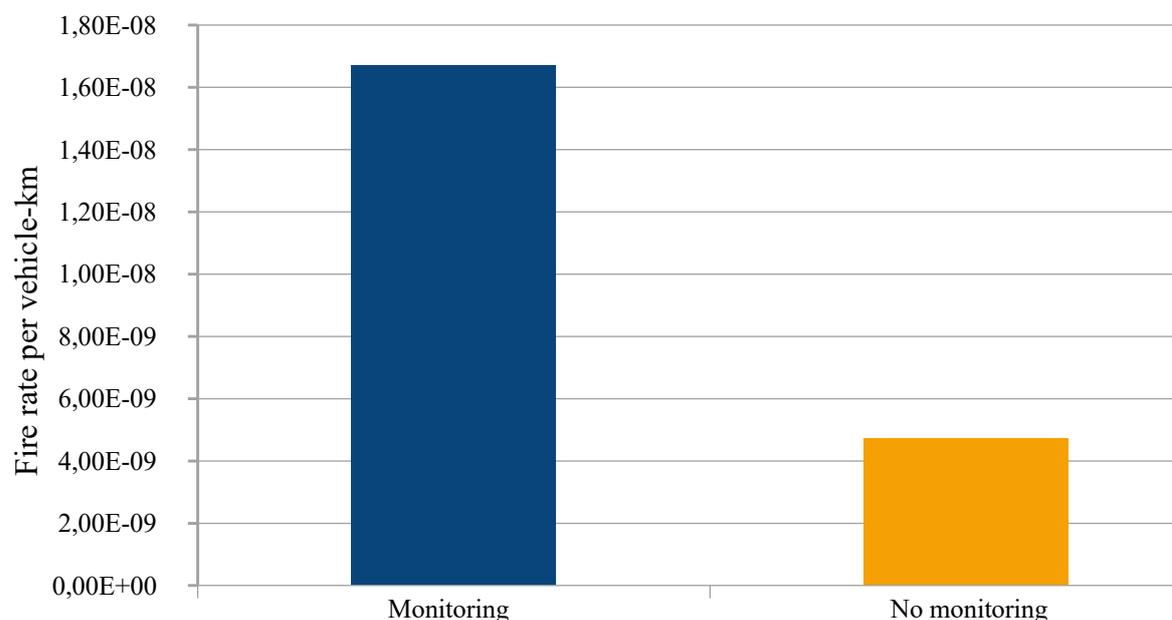
*Illustration 9: comparison of fire rates in tunnels (in norway) with and without monitoring*
